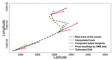
Figure 2. Schematic representation of the comparison between real and interpolated track for three succeeding VMS records towards an estimated one. Spline tangents and vectors are shown.
